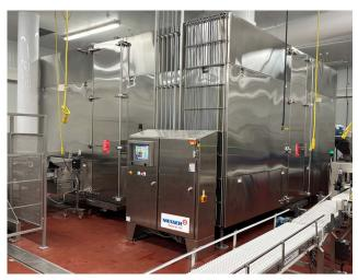
By installing a new, advanced-design Messer spiral freezer, Rhino Foods boosted production of ice cream and ready-to-eat inclusions. The company improved both freezing and labor efficiency in a smaller space.
