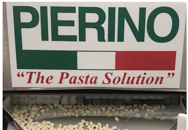
Pierino Gnocchi is pictured entering (top image) and exiting (bottom image) of the Messer Wave Impingement Freezer. The wave-like action helps keep the product separated while the impingement gas flows increase throughput, cryogen efficiency and operating leverage for the premium pasta maker.
